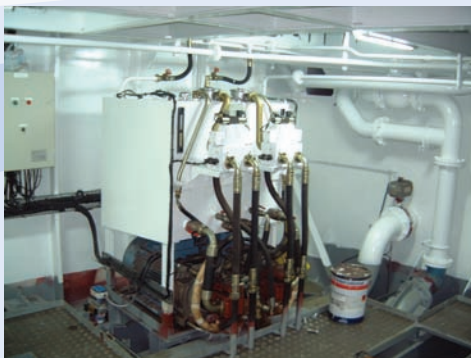
Power pack for steering gear.
