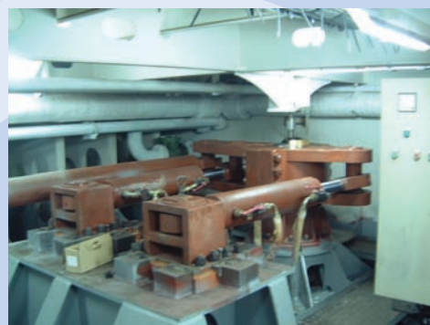
35 T x m steering gear on board.
