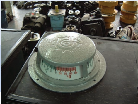
Rudder angle indicator for ceiling mounting, with light.
