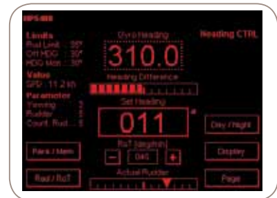
NautoPilot® 5000 main screen with touch operation
